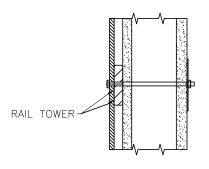
HOLLOW CONCRETE BLOCK, THRU-BOLT WITH 1/2" THREADED ROD
