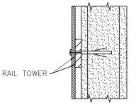
CONCRETE WALL OR FILLED CONCRETE BLOCK, USE 1/2" X 6" CONCRETE ANCHOR
